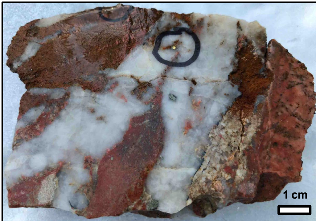
Plate 6-2. Hand specimen of altered syenite hosting stockwork quartz veins containing pyrite + visible gold.
