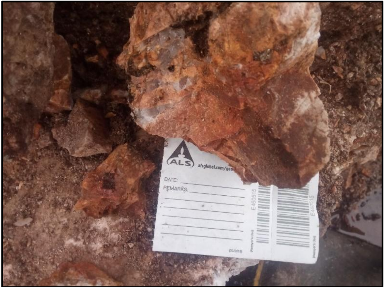
Plate 6-5. Sample photograph of E460515 containing hematite altered syenite with cm-thick quartz veins and coarse-grained pyrite, which returned an assay of 0.978 g/t Au.
